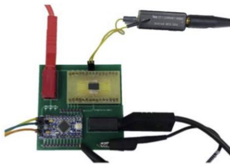
Figure 4: Measurement setup for acquiring power traces from a TMS37126 IC (on the yellow breakout board). Top-right: Tektronix CT-1 current probe. Bottom-left: Arduino Pro Mini functioning as a serial to SPI translator.
