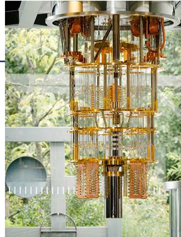
IBM 5Q System: An IBM cryostat wired for a 50 qubit system.
